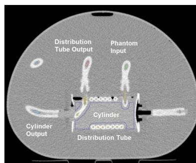
A single axial slice of the dynamic flow phantom submerged in the acrylic shell depicting the manually contoured regions of interest.
