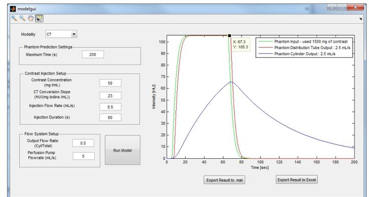
The phantom input and distribution output tube peaks are nearly equal in magnitude to those produced in Case 1; although the amount of contrast agent entering the system is greater in this case, the concentration and flow
