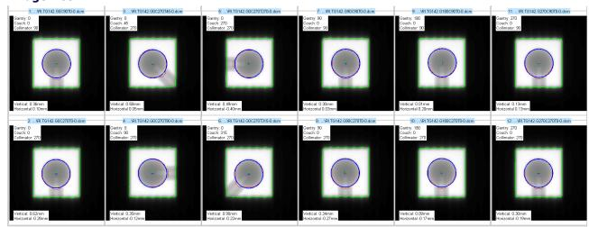
The software calculates and displays both the center point and boundaries of ball and radiation field along with the raw "Horizontal" and "Vertical" displacement for each image.
