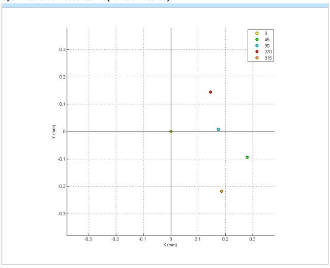
This plot shows couch (table) deviations post-optimization with respect to the gantry and collimator mid-point (Pm) for various couch angles.
