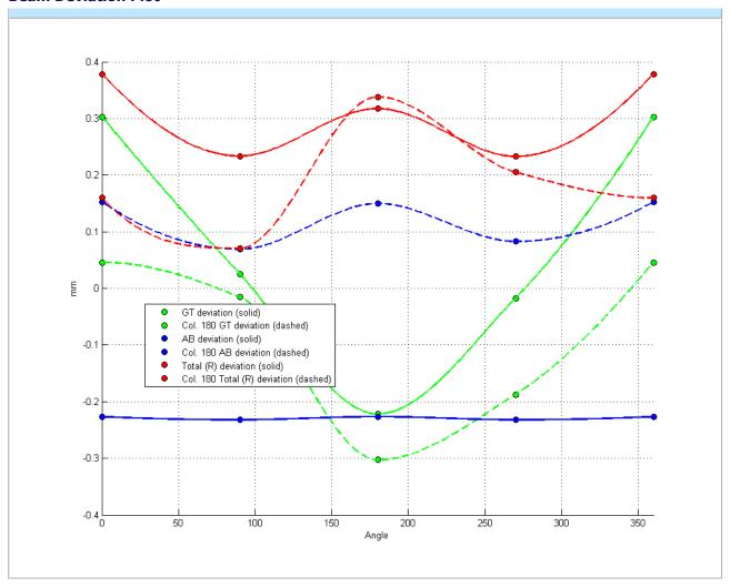
This plot shows the contributions from the gantry and collimator to the isocenter drift. The solid lines and dashed lines represent opposed collimator angles.
