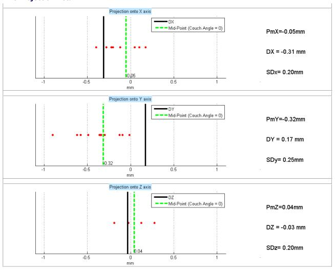
These plots show the ball-Field displacement projections onto the X, Y, and Z axes for all images.
