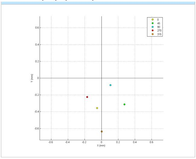
This plot shows couch (table) deviations pre-optimization without ball setup error and with respect to the gantry and collimator mid-point (Pm) for various couch angles.
